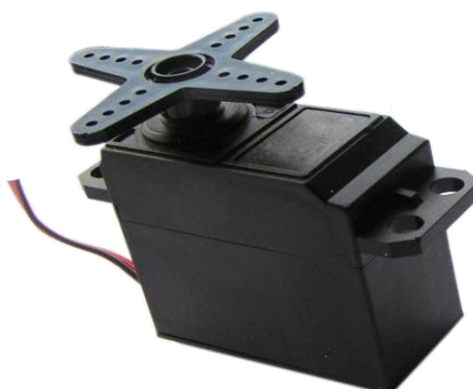
Figure 12. A 5 V d.c Servo motor used for 360 revolution of arm.
